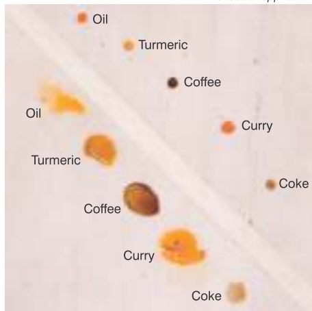
Absorption of stains before application of sealer
